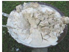
Addition of water = slaking
