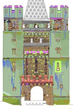
Material and deterioration patterns
