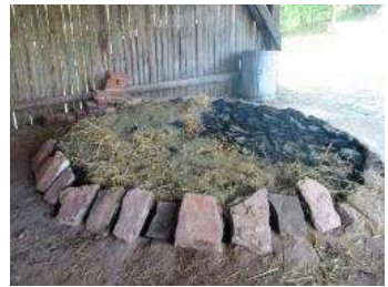
next morning dehydration nearly complete; clay covering is applied
