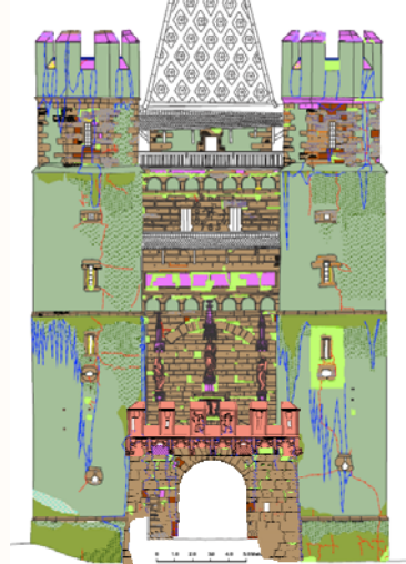
Material and deterioration patterns cartography, CSC juli 2011
